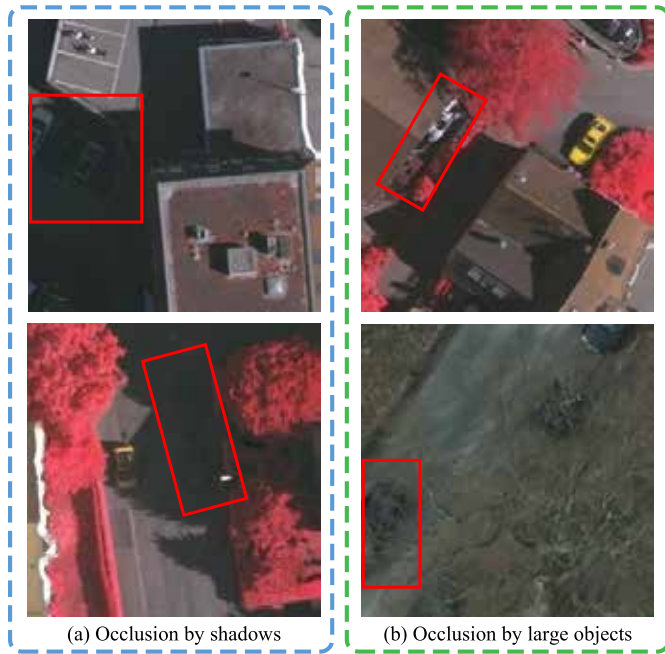
Fig. 1. Exhibit the case where the small objects are occluded. (a) Car is shadowed by the building. (b) Car is obscured by the building or a tree.
